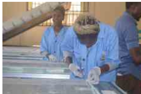
Auxano Staff trimming stringed cells in preparation for panel lamination
