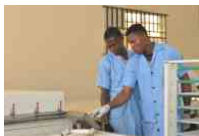
Auxano staff in the process of laminating solar panels
